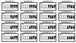
Address 0 is the RTD-20 MASTER address. Address 1 to 15 are RTD-20 SLAVE addresses.
